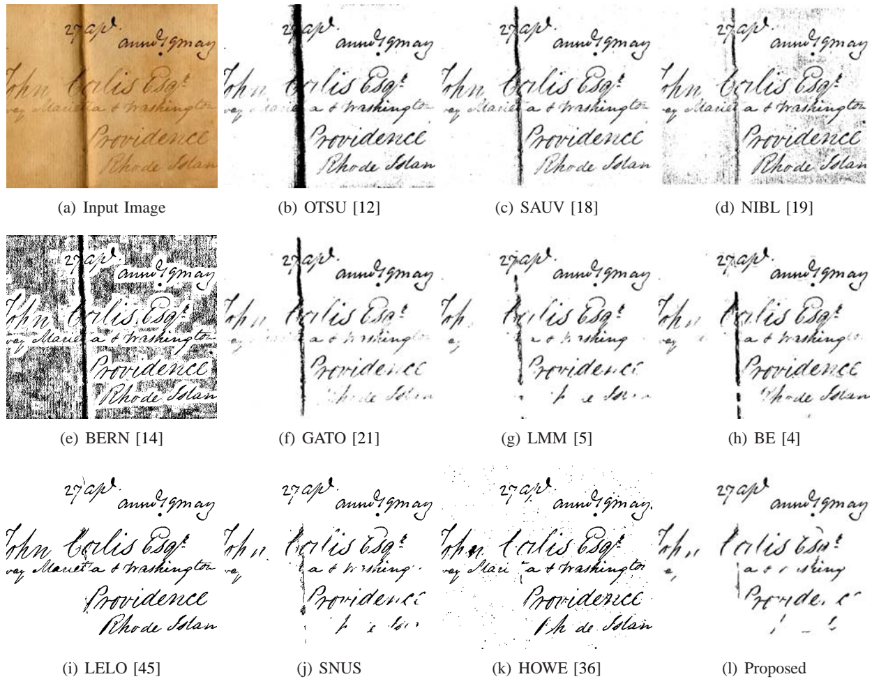
Fig. 13. Binarization Results of the sample document image (HW 06) in DIBCO 2011 dataset produced by different methods.
