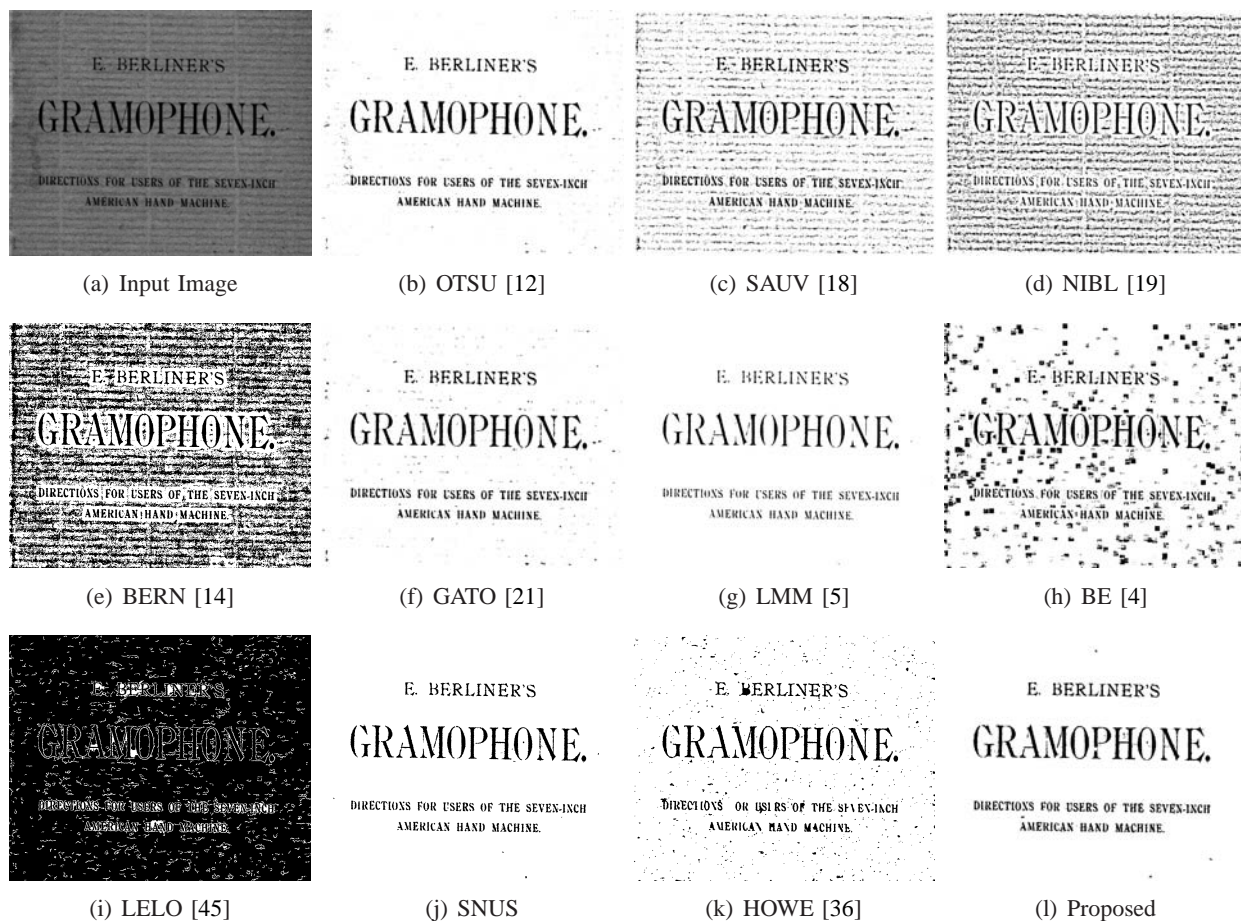
Fig. 11. Binarization Results of the sample document image (PR 06) in DIBCO 2011 dataset produced by different methods.
